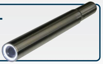
The SC-166 downhole camera is designed for water wells, boreholes and vertical shafts as small as 2 inches in diameter. This camera has effective survey capabilities for 2-inch to 10-inch (5-cm to 25-cm) well diameters. The SC-166 well camera system comes equipped with a protective carry case provided for storage, adjustable centering bands, and cable head protector.
