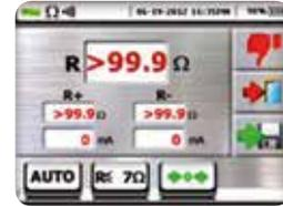
Continuity of protective conductors: Measurement result negative
