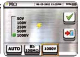
Selection of test voltage and minimum limit value on MQ measurement
